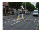
4. *Humps*. TfL preferred them where there is high-speed traffic. However they damage vehicles, affect emergency service response times. If they are installed, the preference is for them to be built at a maximum height of 75mm.
